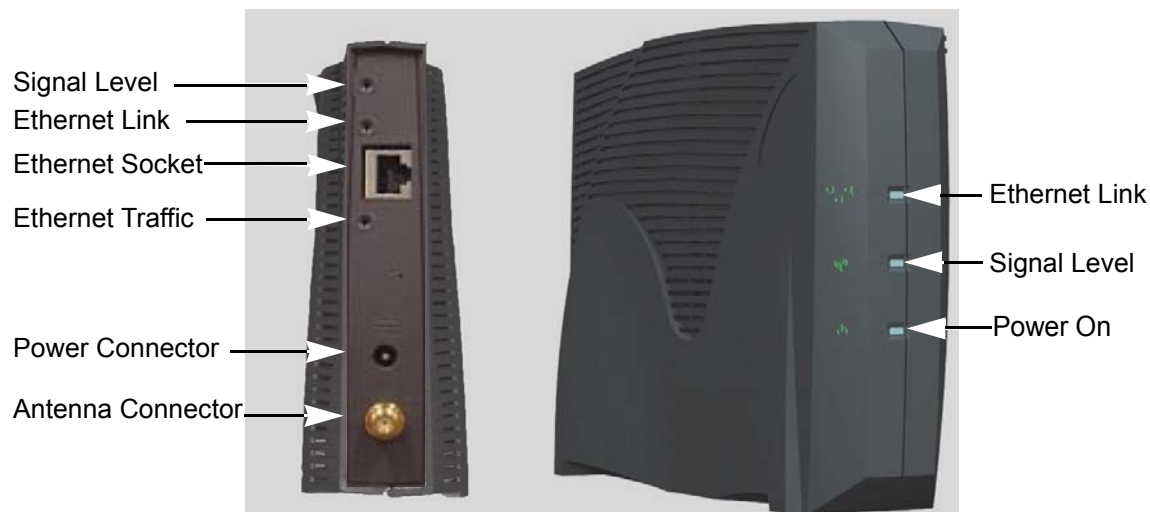
Figure 6 EUM3005 Modem - External Indicators and Connectors
