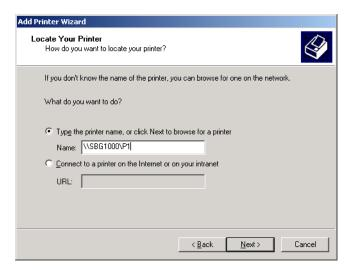
32 In the Type the printer name,... field, type \\Print Server Name\Queue Name and click Next. It must match the Print Server Name\Queue Name set on the SBG1000 Printer > CONFIGURATION — Microsoft smb Page (see page 82). The default is \\SBG1000\P1.
