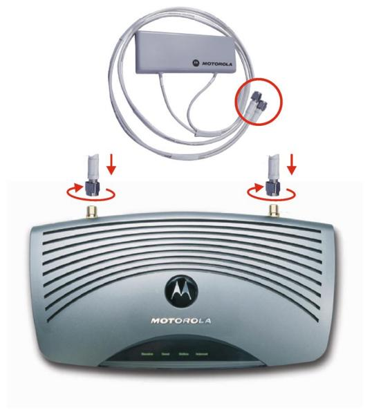
4 Position or mount the External Diversity Antenna in a suitable location away from the computer and monitor. Follow the instructions provided with the External Diversity Antenna. Do not twist the antenna cables.
