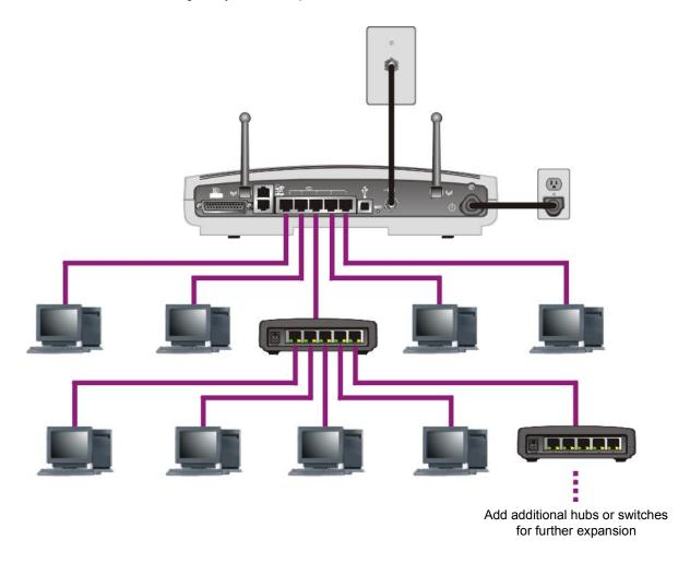
You can connect a hub or switch to any Ethernet port on the Motorola SBG1000 Wireless Cable Modem Gateway.
