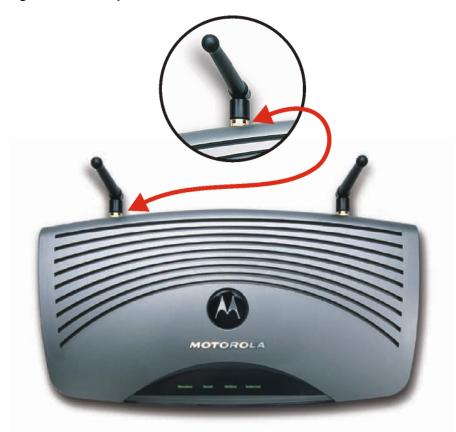
3 Connect the cables from the Motorola External Diversity Antenna to the connectors on the Motorola SBG1000 Wireless Cable Modem Gateway Front Panel. Hand-tighten the connectors to avoid damaging them. Using excessive force may damage the connectors.
