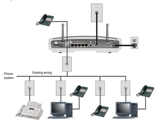
Each computer requires an HPNA adapter to connect to the HPNA network. HPNA adapters (sold elsewhere) are available for PCI or USB. After installing the HPNA adapter, you must install HPNA driver software on the computer following the instructions provided with the HPNA adapter.
