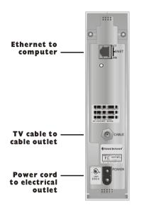
You must call your service provider to activate your service. You need to provide the media access control (MAC) address. This address is found on the barcode label marked HFC MAC ID on the rear panel. The address format is 00:20:40:xx:xx:xx.
