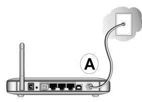
Figure 3-1: Connect the gateway to the cable network.
