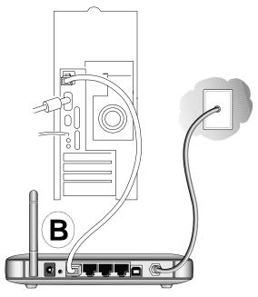
Figure 3-2: Connect a PC to the gateway
