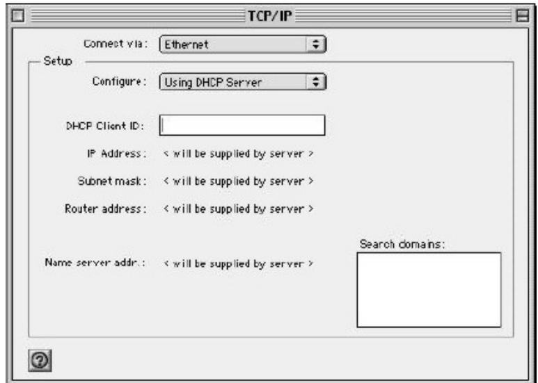
3. For dynamically assigned settings, select **Using DHCP Server** from the **Configure:** list.
