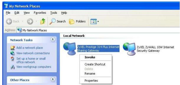
**Step 6.** Right-click the icon for your ZyXEL device and select **Properties**. A properties window displays with basic information about the ZyXEL device.
