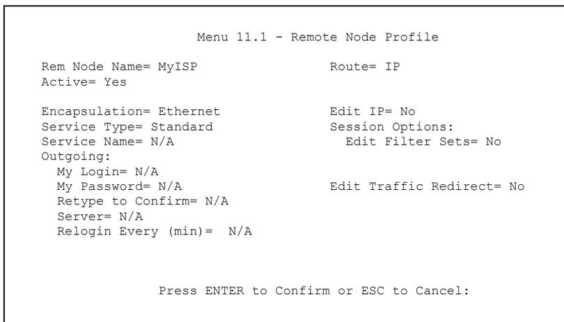
**Figure 25-1 Menu 11.1 Remote Node Profile for Ethernet Encapsulation**
