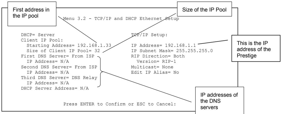
**Figure 23-3 Menu 3.2 TCP/IP and DHCP Ethernet Setup**
