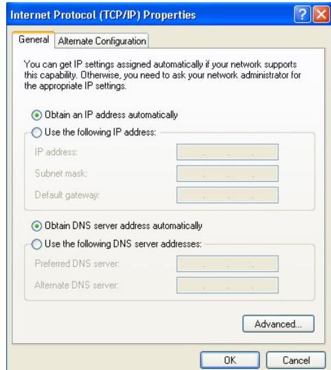
6. -If you do not know your gateway's IP address, remove any previously installed gateways in the **IP Settings** tab and click **OK**.
