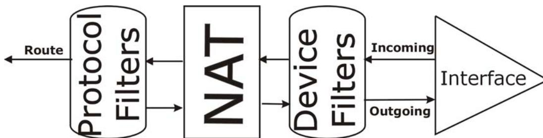
Figure 30-12 Protocol and Device Filter Sets
