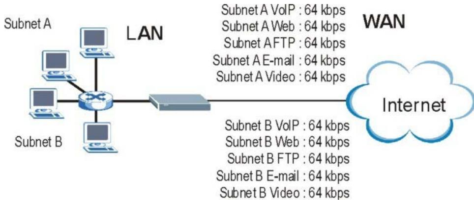
**Figure 18-3 Application and Subnet-based Bandwidth Management Example**
