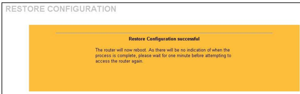
**Figure 19-11 Configuration Restore Successful**
