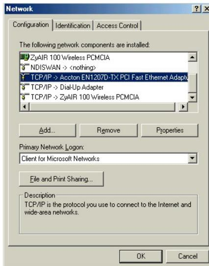
2. The **Network** window **Configuration** tab displays a list of installed components. You need a network adapter, the TCP/IP protocol and Client for Microsoft Networks.
