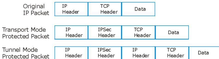
**Figure 15-3 Transport and Tunnel Mode IPSec Encapsulation**
