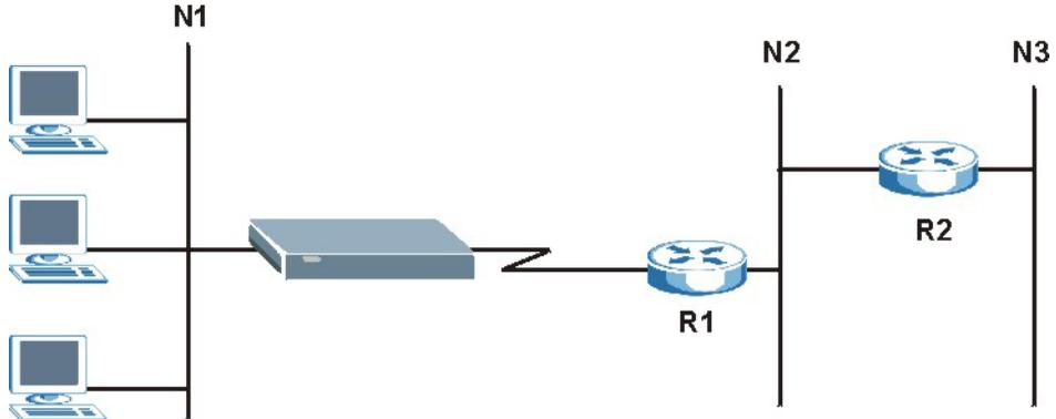
Figure 11-1 Example of Static Routing Topology
