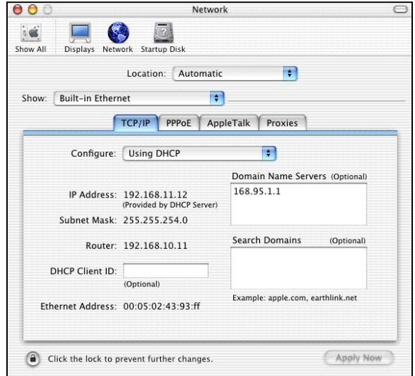
3. For dynamically assigned settings, select **Using DHCP** from the **Configure** list.
