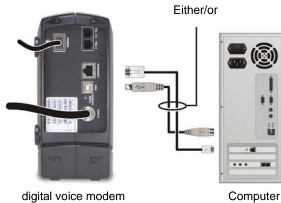
**USB:** Be sure the SURFboard Voice Modem CD-ROM is inserted in your CD-ROM drive. Perform the appropriate procedure for [Setting Up a USB Driver](#) for your Windows version. Connect the USB cable to the USB port on the digital voice modem. Connect the other end to the USB port on your PC.
