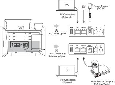
Note: The IP phone should be used with Yealink original power adapter (5V/2A) only. The use of the third-party power adapter may cause the damage to the phone. If you are connecting a PC to your phone, we recommend that you use the Ethernet cable provided by Yealink. If inline power (PoE) is provided, you don't need to connect the power adapter. Make sure the hub/switch is PoE-compliant.
