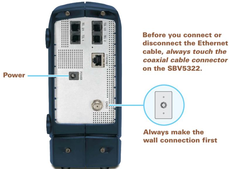
**Before you connect or disconnect the Ethernet cable, always touch the coaxial cable connector on the SBV5322.**
